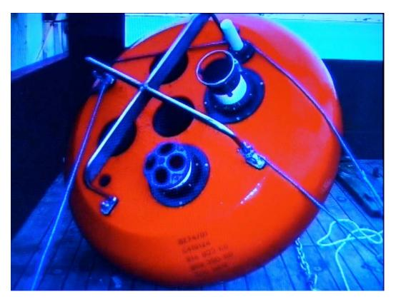
which carries the instruments, and once the weight was settled on the bottom the buoy was submerged by about 200 metres and was carrying out current speed and direction measurements above the buoy and also measuring the plankton, hopefully krill, in the water column above the buoy.
