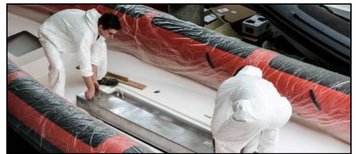
▲ Fitting the under-deck stainless steel fuel tanks
