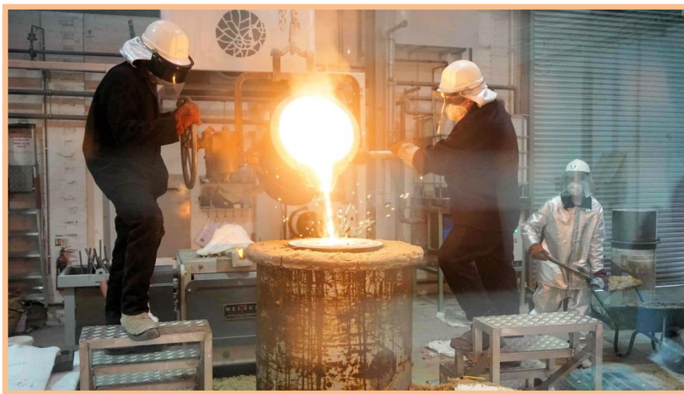
(Stainless steel casting of the Antarctic Monument at temperatures in excess of 1600° C – photo Rod Rhys Jones)
