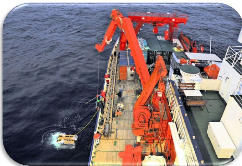
(The ROV being launched from RV Meteor)
